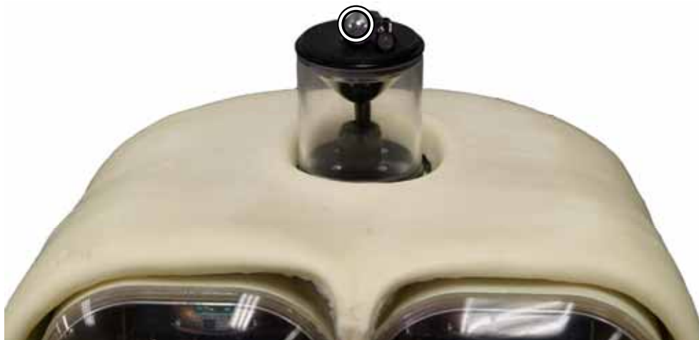
Figure 3. A microphone, attached on a omni-directional mirror, is located on top of the head
